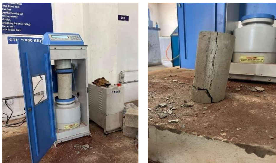
Fig.5.2 splitting tensile strength test on cylindrical specimen
