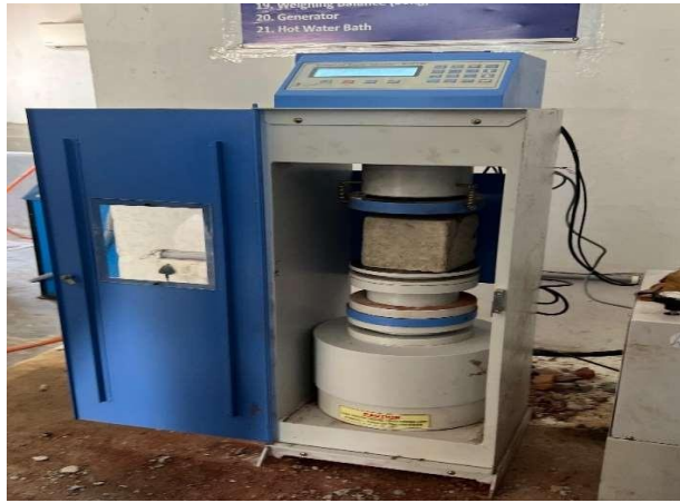
Fig.5.1 compression testing on cube specimen
