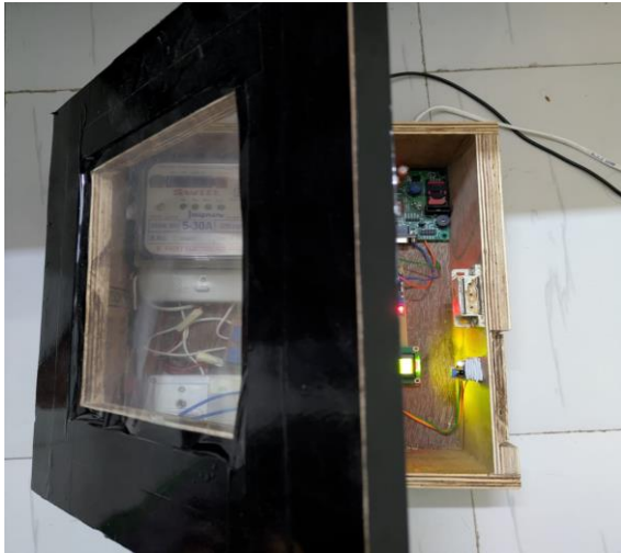
Figure 7.1.5: casing on electricity meter to detect theft
