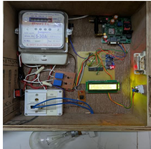
Figure 7.1.6: Electricity Cut when theft detected
