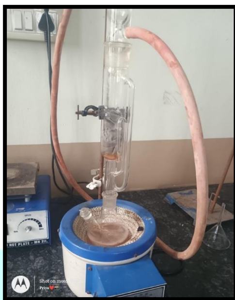
Fig.1- Extraction of Ashoka Bark by Soxhlet Appartaus
