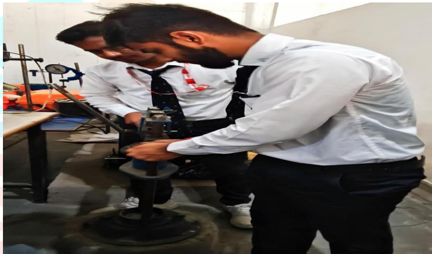
Aggregate impact value test done by project member
