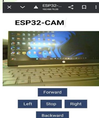
Fig 7 Dashboard of ESP32 Wi-Fi Controlled Car with Live Camera
