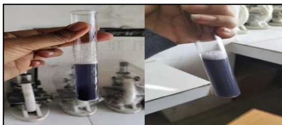
Fig. no.6: Dirt dispersion test
