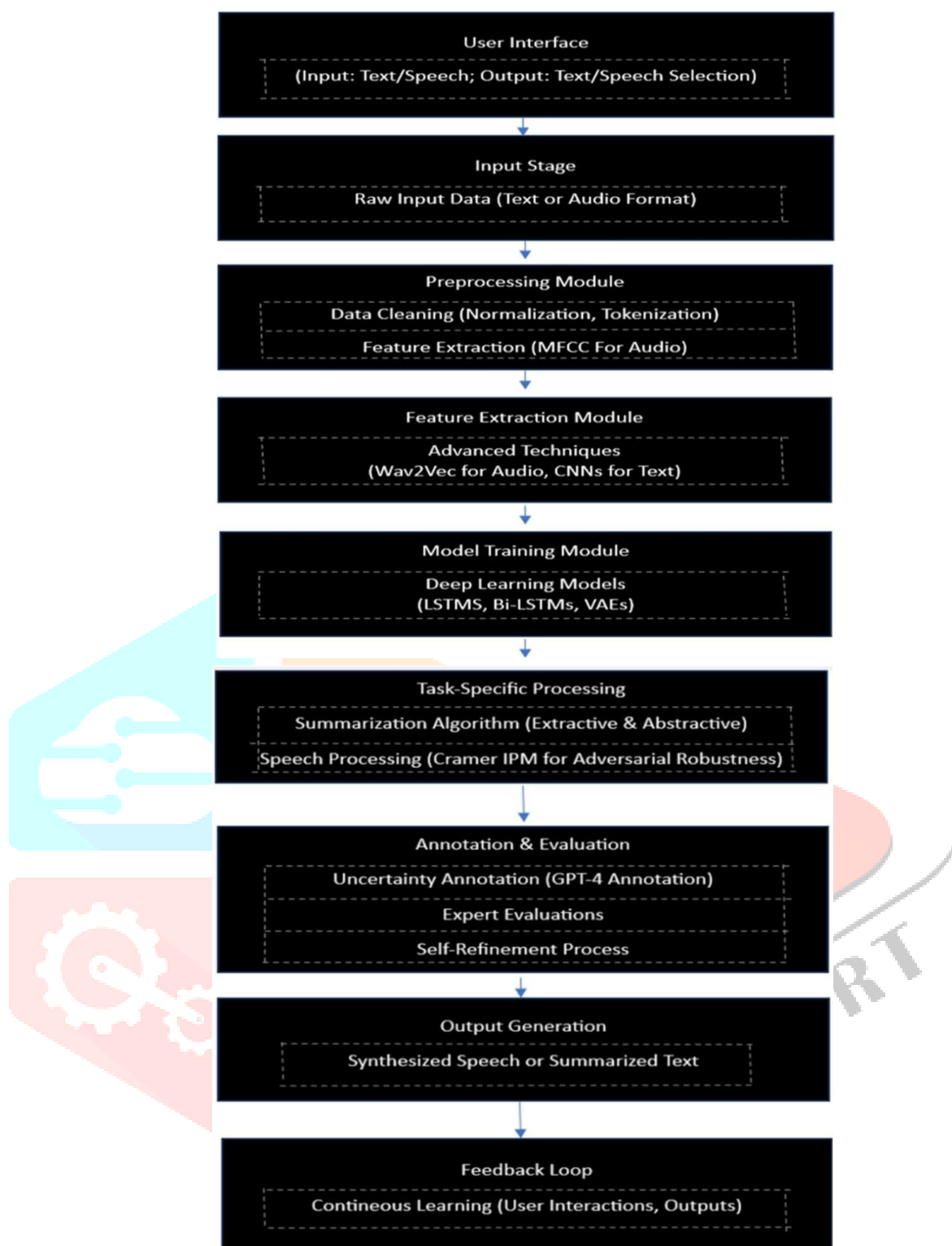
FIG 1 PROCESS FLOW OF MULTIMODAL TEXT AND SPEECH CONVERSION WITH SUMMARIZATION
