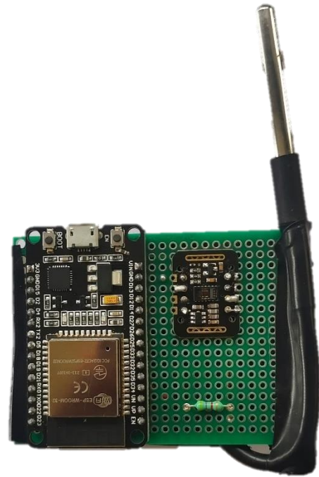
Fig 1: Iot Device integrated with sensors
