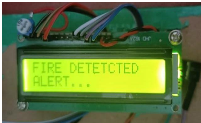
Fig 5: Fire detected alert message comes through message the display unit
