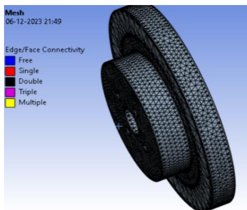
Figure 4: Tetrahedral mesh disc brake
