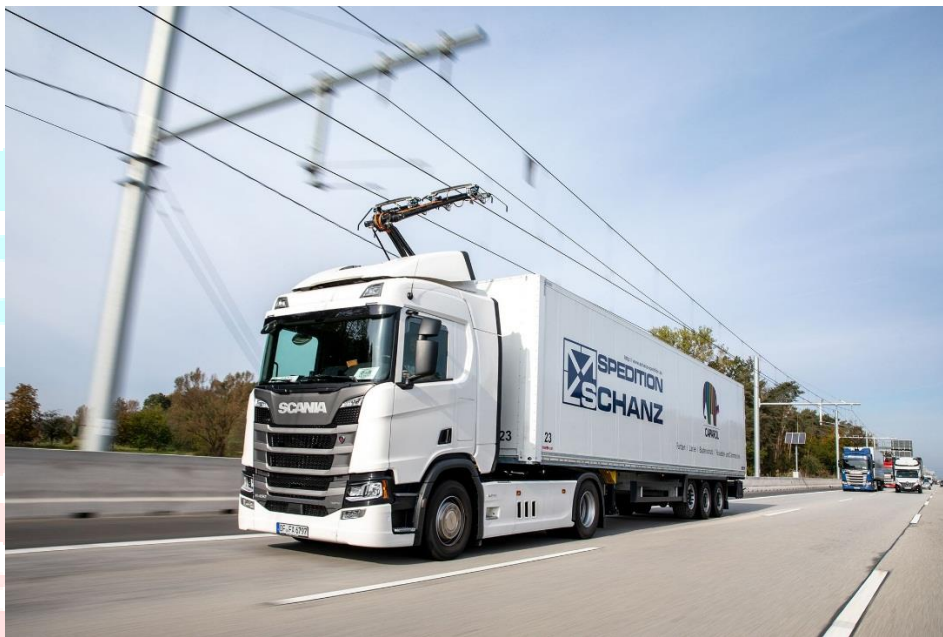
Fig-1 Illustrates a truck driving on an electrified road using overhead lines.
