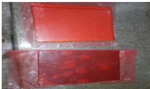
Figure 2. (a) Pre-Compaction Laminates Figure 2. (b) 10mm and 12 mm thickness cured Laminates
