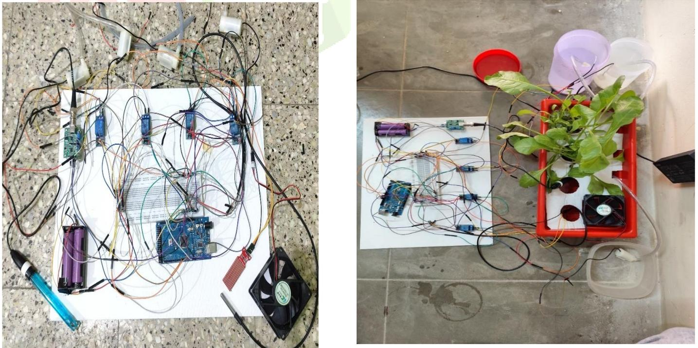
Fig 2: Automated hydroculture monitoring system
