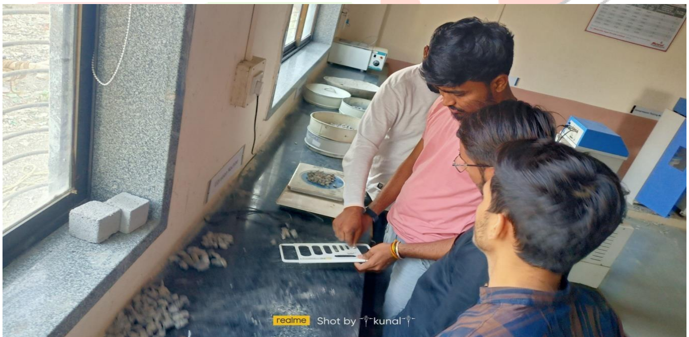
Image 3 :- Team Members Performing Flakiness Index Test
