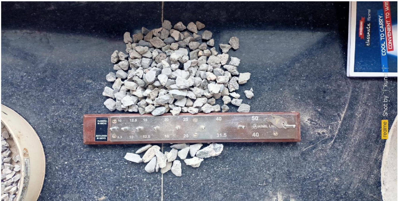
Image 4 :- Elongation Test Performed
