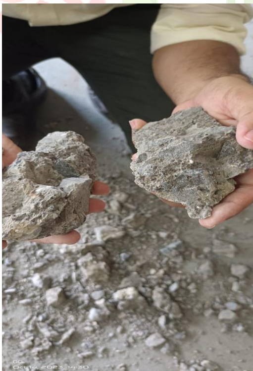
Image 6:- Compression Test Performed On Cube
