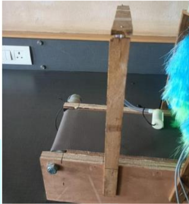
Fig. 8. Vehicle detection and activation of Pump for Pre-wash
