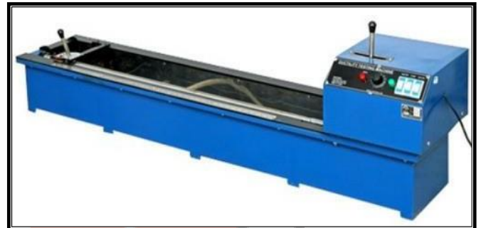
Fig 7: Ductility Test Apparatus
