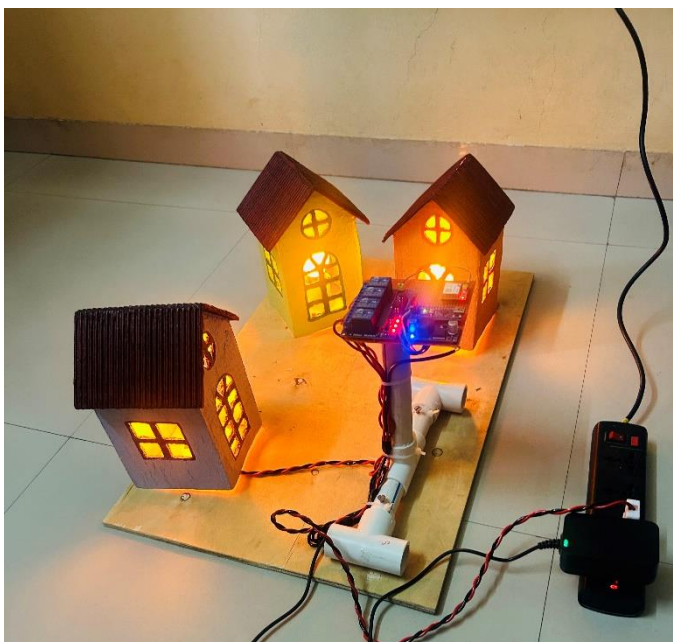
Fig. 5 Proposed System Hardware – ON condition
