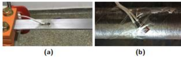
Figure 8: Strain- gauges glued to the analyzed mechanical system (8a) in experiment 1 and (8b) in experiment 2.
