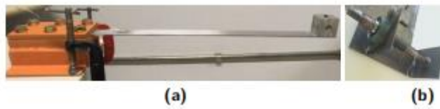
Figure 7: Test benches for experimental validation of the proposed measurement system: (7a) Cantilever beam and (7b) Crimped-supported shaft under torsion.
