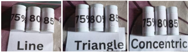
Fig.8 (a) Fabricated Compression test Samples (layer thickness 0.1 mm)
