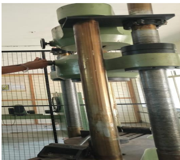
Fig. 6. Schematic of tensile testing equipment (Universal testing machine).
