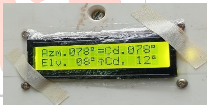
Fig. 1.5: Azimuth feedback value made equal to command value
