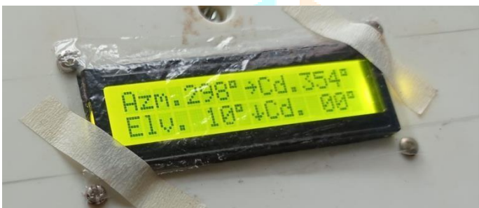
Fig. 1.12: Input value obtained through Orbitron displays on LCD
