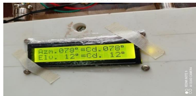
Fig. 1.6: Elevation feedback value made equal to command value
