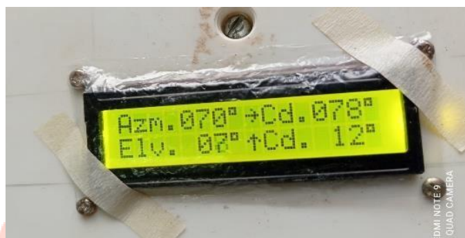
Fig. 1.4: Input value fed through encoder displays on LCD
