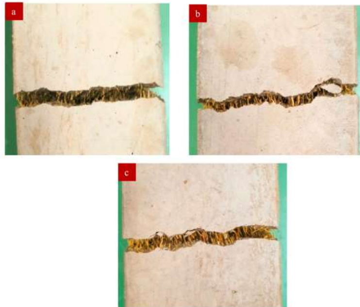
Figure 8 Failure pattern (a) 4% (b) 6% (c) 8% bamboo fibers
