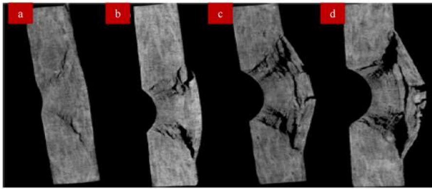
Figure 14 Varying diameter of pits as the impact energy increases
