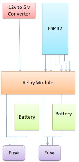
**Converter(12v to 5v):** A voltage converter that steps down from 12 volts (V) to 5 volts (V) is commonly referred to as a DC-DC buck converter. Buck converters are widely used in electronics to efficiently reduce voltage levels while maintaining a stable output.
