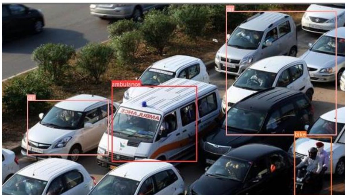
Figure 8. Ambulance is detected among other vehicles on the road according to the various object classes provided to the model
