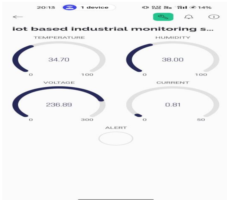
Fig 9: Results of voltage, current levels using Blynk iot
