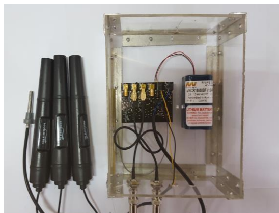
Fig. 3: Deployment Setup with the sensors and Waspnote microcontroller board.
