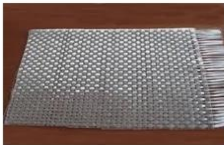
Fig 2.1: Cut pieces of woven e-glass 350 gm glass fiber.
