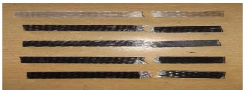
Fig 2.4: Tensile test done on the specimens.
