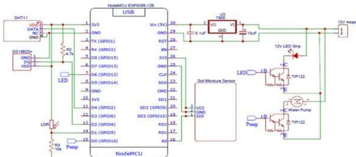
**Fig 1: Circuit Diagram of Green IOT solutions for Intelligent farming**
