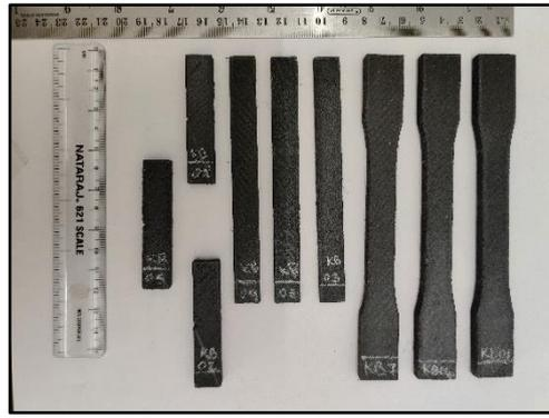
Fig.2 Printed Specimens of PETG
