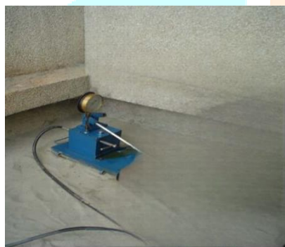
Fig 2. Loading from hydraulic jack
