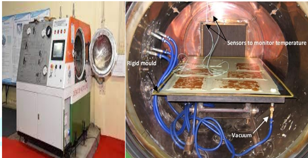
Fig.4: Stages of vacuum bagging hand lay-up processes
