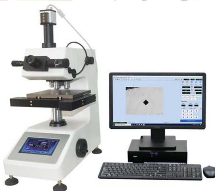
Fig.13: Set-up in lab for conduction of micro Vicker's hardness test on the specimen
