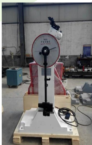
Fig.15: Izod impact testing set-up used for conducting the test
