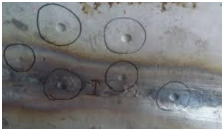
Fig. 14: Specimen showing the indentation markings
