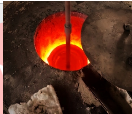
Figure 2. Mechanical Stirrer in molten metal
