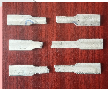
Figure 15 Stir casted specimens after tensile test
