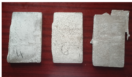
Figure 5. Composite samples after removing from the die
