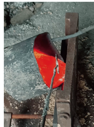
Figure 4. Pouring molten metal into the die
