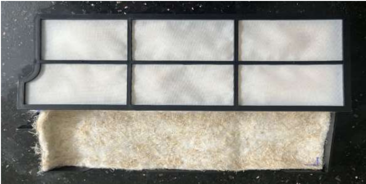
Fig 4.1. AC filter using sisal and recycled polyester fiber
