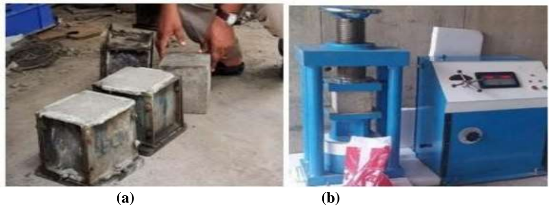
Figure 3.8 (a) Cube specimen demoulding and (b) Cube failure mode
