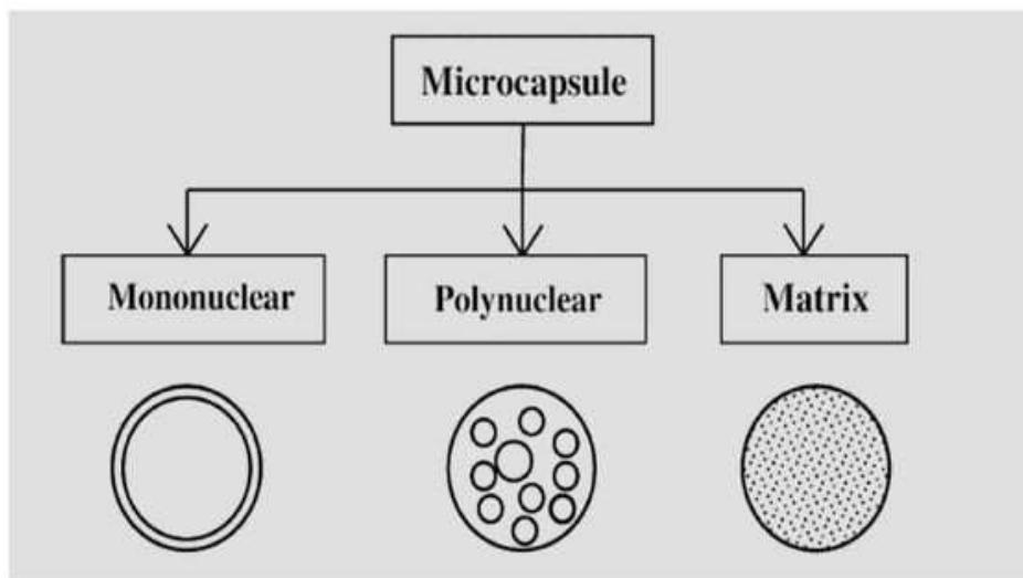
Microcapsule morphology is mostly determined by the shell's deposition mechanism and core substance monomers.
