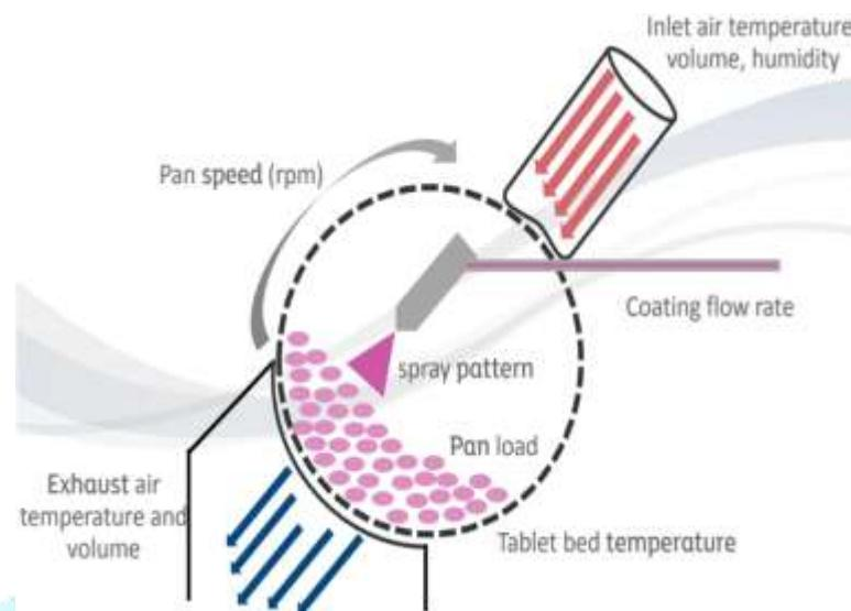
The pan coating technique, widely employed in the pharmaceutical sector, is one of the oldest industrial procedures for producing small coated particles or tablets. The particles are tossed in a pan or other device while the coating material is applied gradually. The pan coating technique, widely employed in the pharmaceutical sector, is one of the earliest industrial procedures for creating small, coated particles or tablets.
