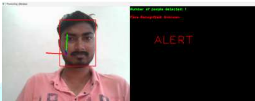
Fig. 9. Output from Face Verification module for frame with invalid examinee.
