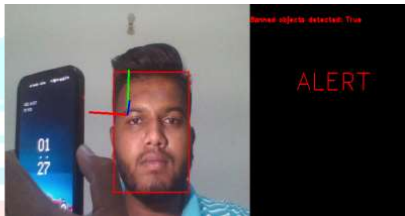
Fig. 7. Output from Object Detection module for frame with banned object.
