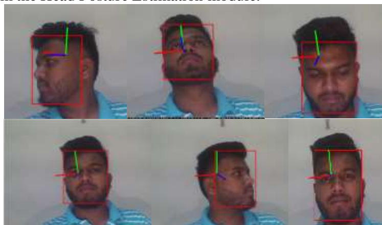
Fig. 13. Output from Head Pose Estimation module. 3D (red, green and blue) vectors are used to illustrate the predicted head pose angles (pitch, yaw and roll)
