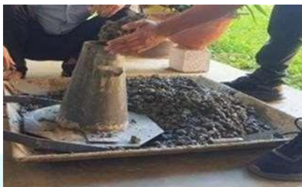
Fig.6: Slump Cone Test
