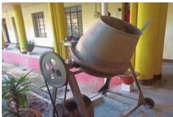
Fig.3: Concrete Mixing Machine
