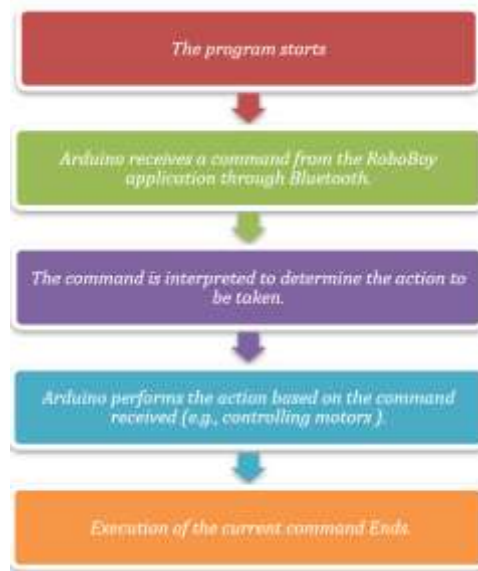
Fig. 4. Flowchart of implemented Robotic Arm
