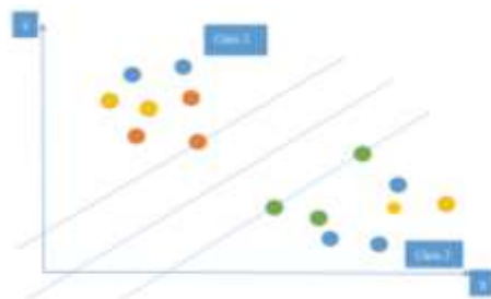
Fig-2- SVM between two classes with the highest margin hyper plane
