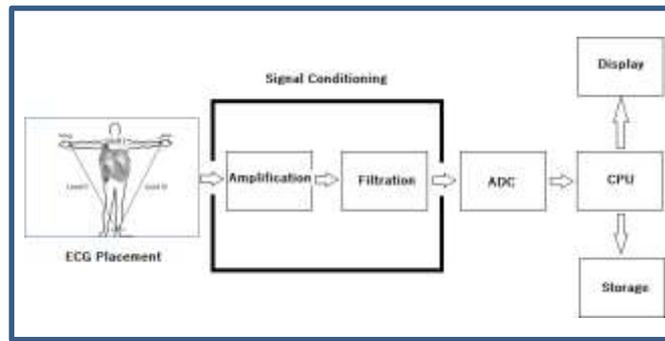
Fig 1. ECG Block Diagram
