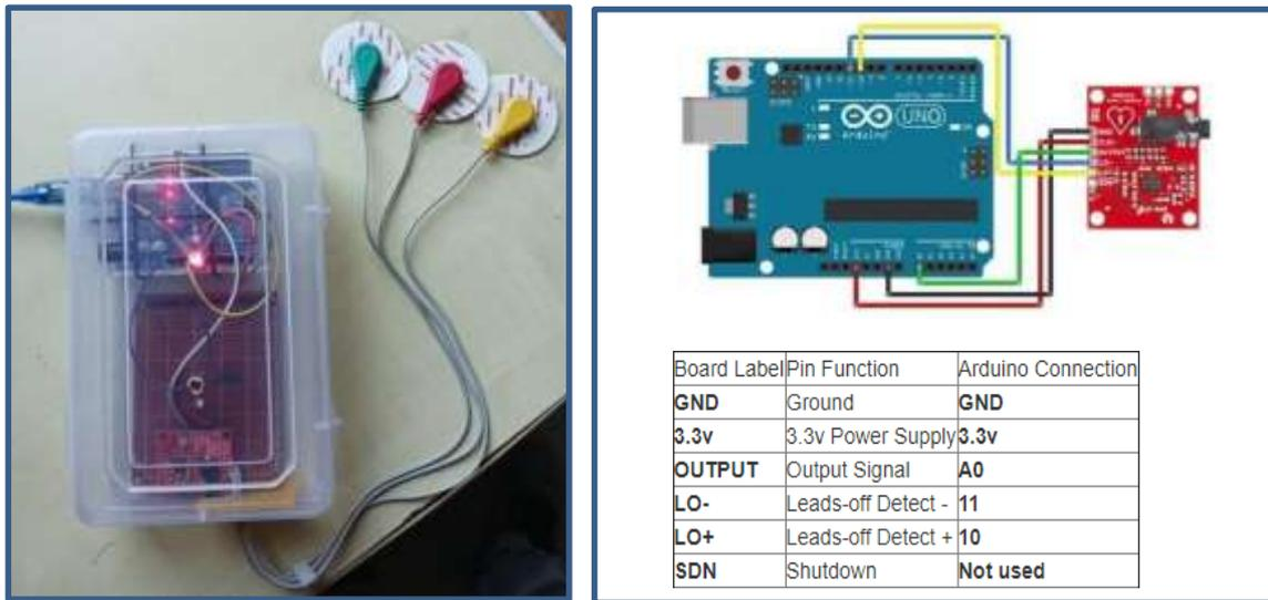
Fig 3. Arduino Uno connected to AD8232
