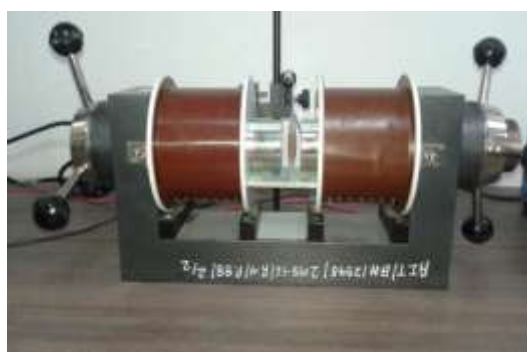
Fig. 1: Electromagnetic field generator with variable magnetic field strength
