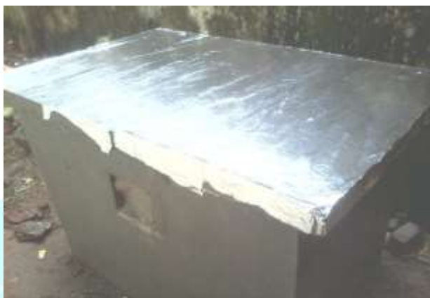
Figure: 2 -Prototype roof blanketed with Aluminum foil
