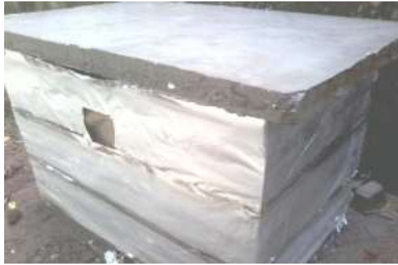
Figure 5-Prototype wall blanketing with aluminum foil
