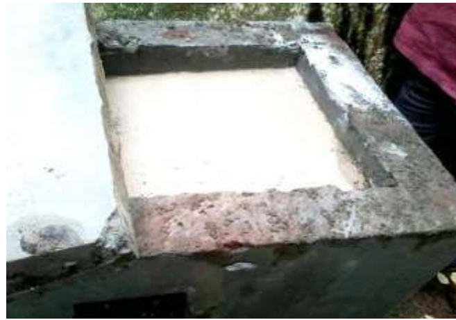
Figure 24 – Prototype with gypsum board false ceiling
