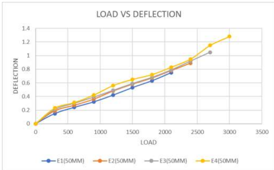
Figure 5.8 Variation Deflection against load for 50mm with different layer of mesh curves.
