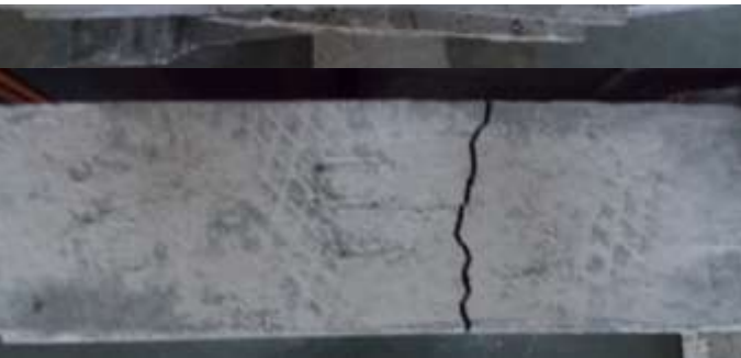
Top view of crack pattern for 40mm thick panel
