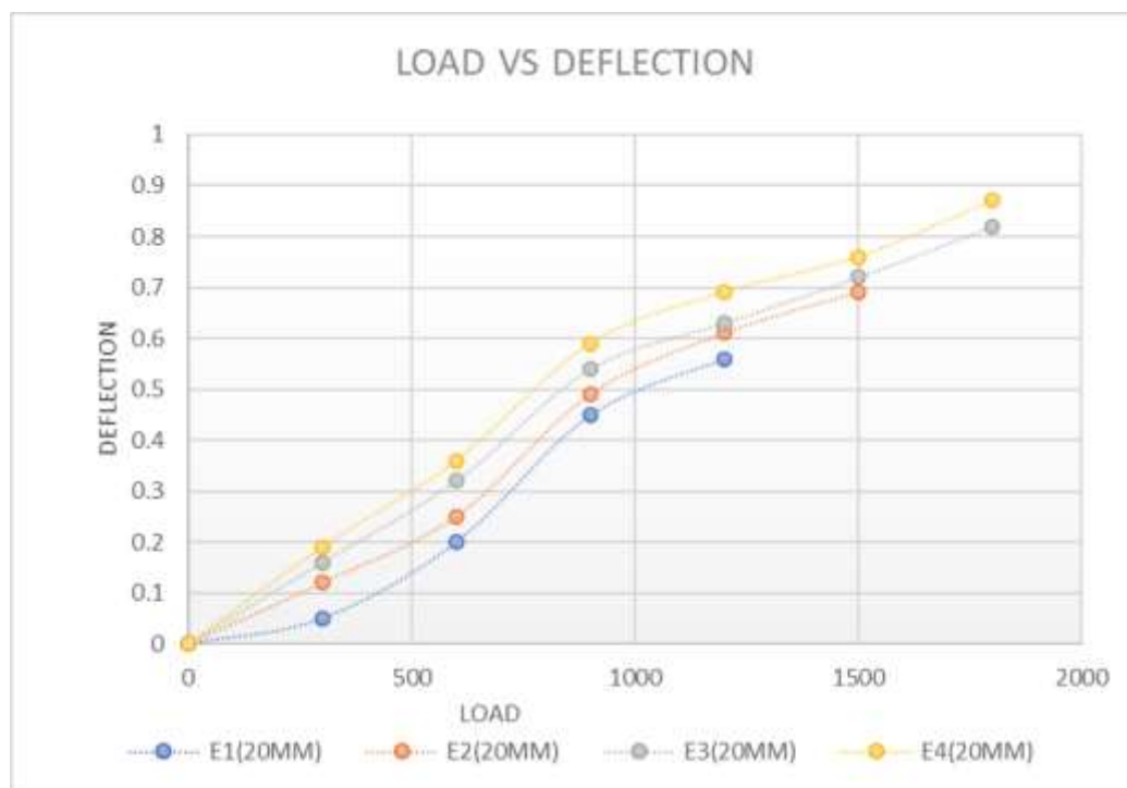
Figure 5.1 Variation Deflection against load for 20mm with different layer of mesh curves .
