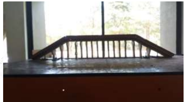
Figure-3 Model fixed on vibration table
