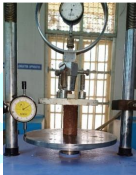
Figure 1 Before failure of UCS soil
