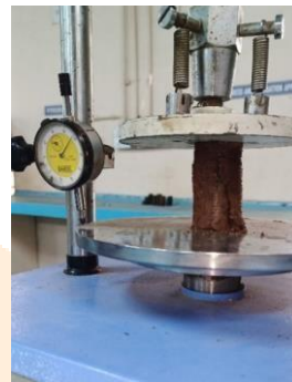
Figure 2 After failure of UCS soil
