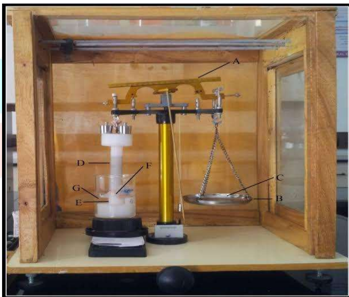
Figure 1. Modified analytical balance used for the Mucoadhesion test.
