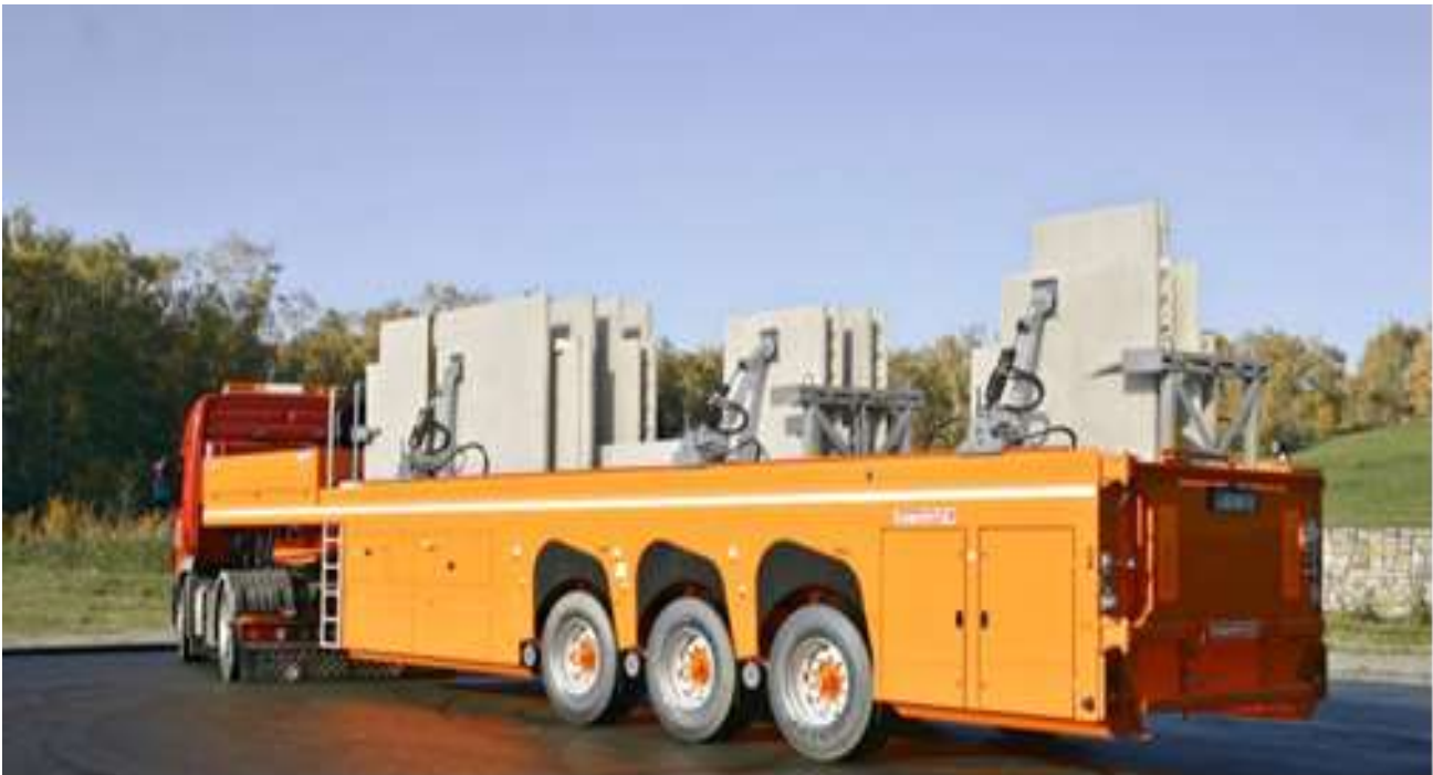
Fig.5 Delivery of Precast Members by Trailor
