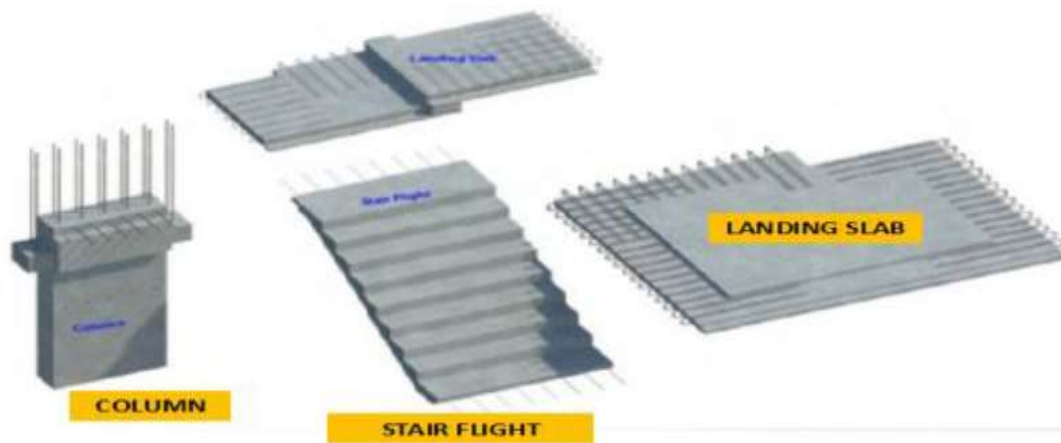
Fig.8 : Precast Column, Staircase and Landing
