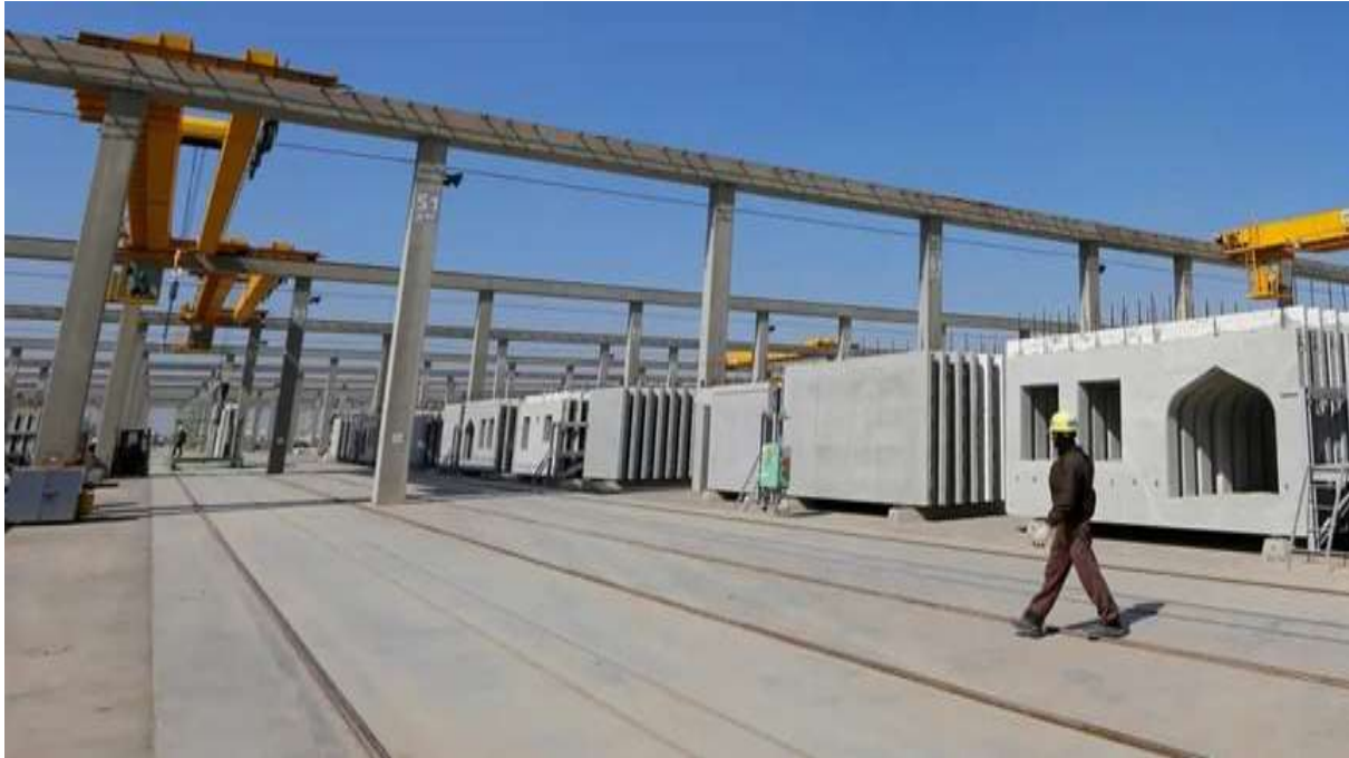
Fig.6 Stacking of Precast Elements at Factory
