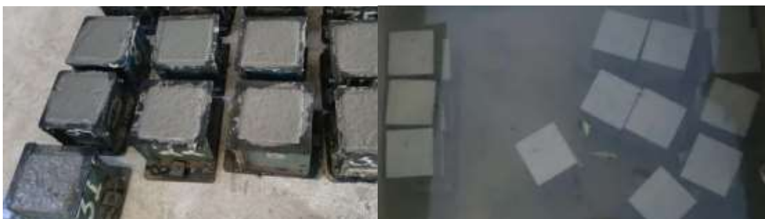
Fig.: Casting Cubes and Curing
