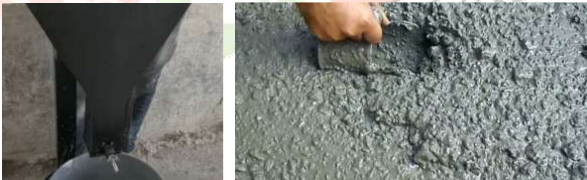
Fig.: V- Funnel Test Equipment and SCC
