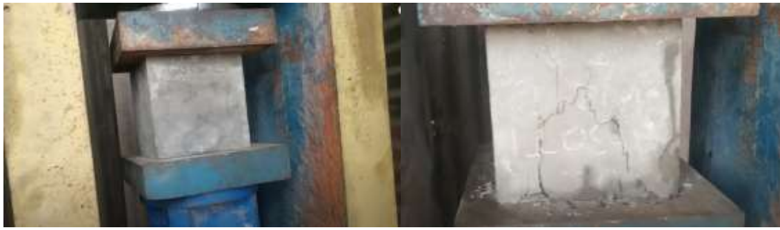
Fig.: Testing of Cubes and Cracks
