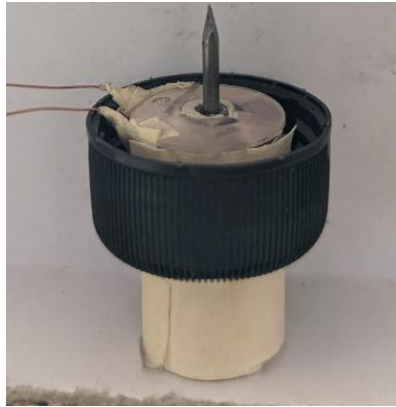
Fig.8: solenoid coil with 442 turns of copper wire
