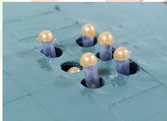
Fig.10: braille character y using solenoids
