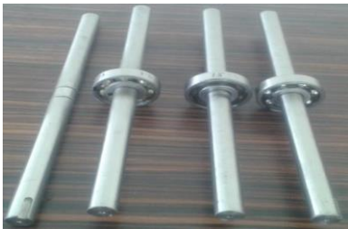
Figure 2: Shaft with Test Bearing
