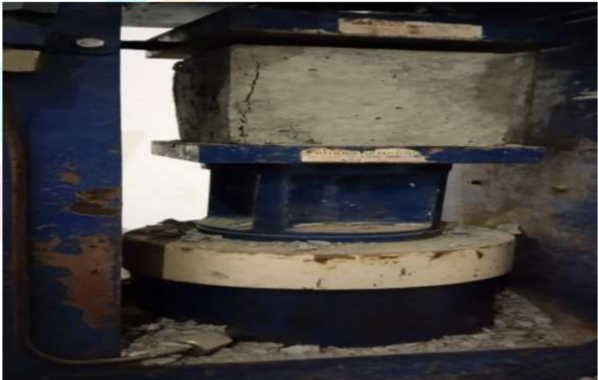
Fig: Testing of concrete cube using CTM
